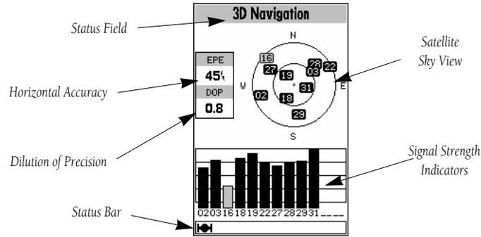
The GPSMAP 130's **status page** provides a visual reference of satellite acquisition and receiver status, with a signal strength bar graph and a satellite sky view in the center of the page. Each page of the GPSMAP 130's system also features an options page, which gives you access to other functions and features that relate to the specific page you are viewing. To get a feel for how the options pages work, lets put the GPSMAP 130 into simulator mode.
