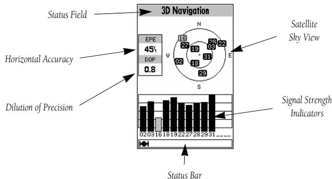
The GPSMAP 130 **status page** provides a visual reference of various receiver functions, including current satellite coverage, receiver operating mode and current receiver accuracy. The status information will give you an idea of what the receiver is doing at any given moment.
