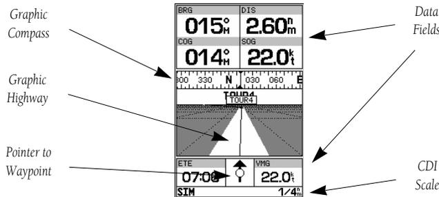
The navigation page provides graphic steering guidance to your destination. The **bearing (BRG)** and **distance (DIS)** to the destination, with your current **course (COG)** and **speed over ground (SOG)**, are displayed at the top of the page, along with a graphic compass to indicate your cardinal heading. The **estimated time enroute (ETE)** and **velocity made good (VMG)**, or the rate you are closing in on your destination) are displayed at the bottom of the page.
