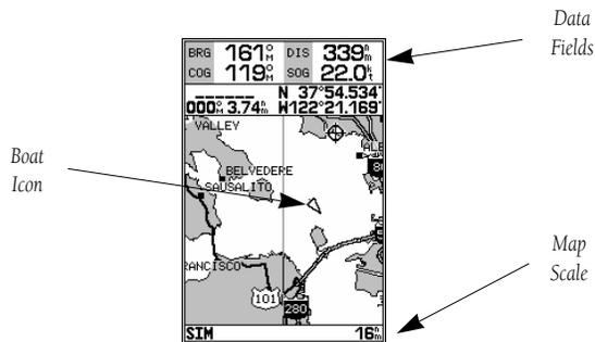
The **map display**, located in the middle of the page, shows your boat as a triangle marker on an electronically generated chart, along with geographic names, markers and buoys that are provided by the G-chart cartridge you're currently using. It also displays your track, routes and nearby waypoints. An on-screen **cursor** lets you pan to other map areas, determine the range and bearing to a position, and perform various waypoint and route functions.
